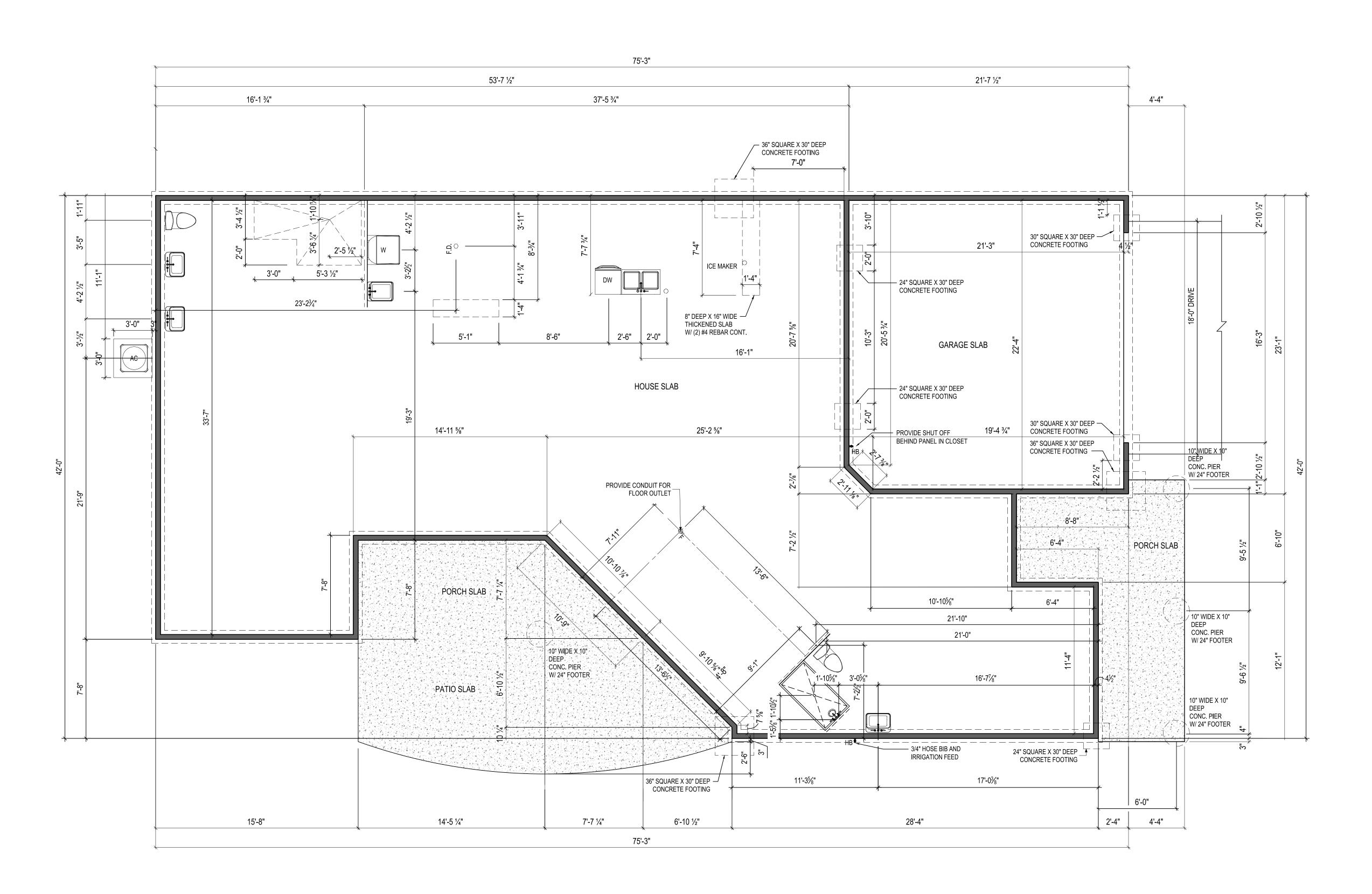
NOTES: THICKENED SLAB SHALL BE REINFORCED WITH CONTINUOUS (2) #4 REBAR
