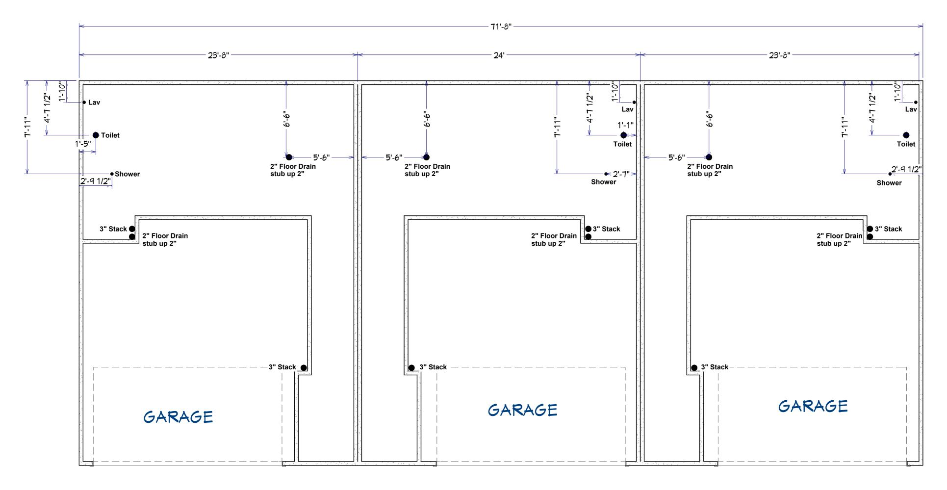
**3" STACK IN GARAGES NO BACKWATER VALVES REQUIRED STUB SEWER AND WATER OUT GARAGE**
