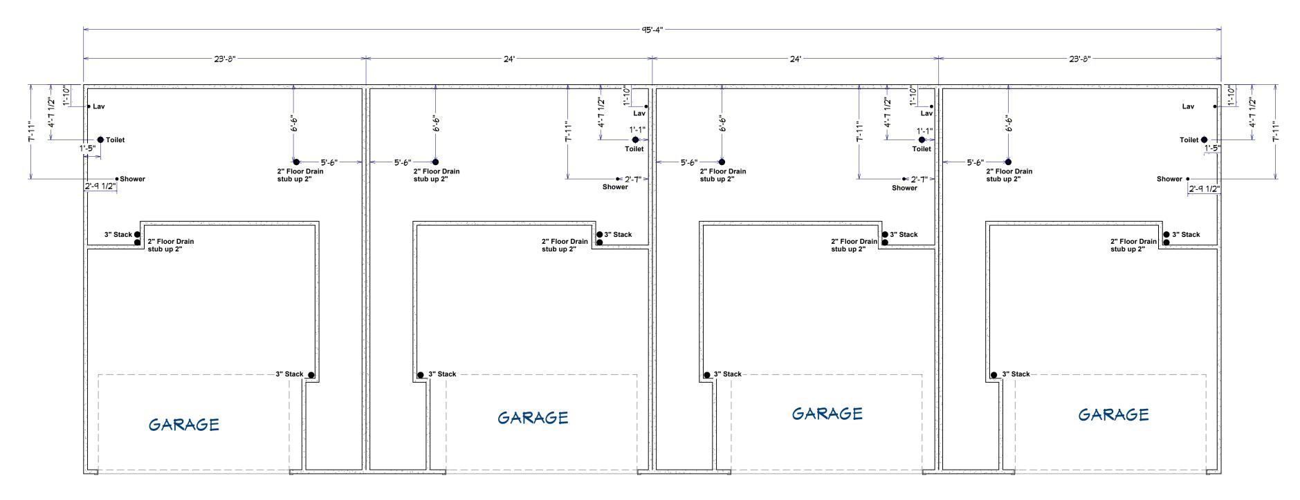
3" STACK IN GARAGES NO BACKWATER VALVES REQUIRED STUB SEWER AND WATER OUT GARAGE
