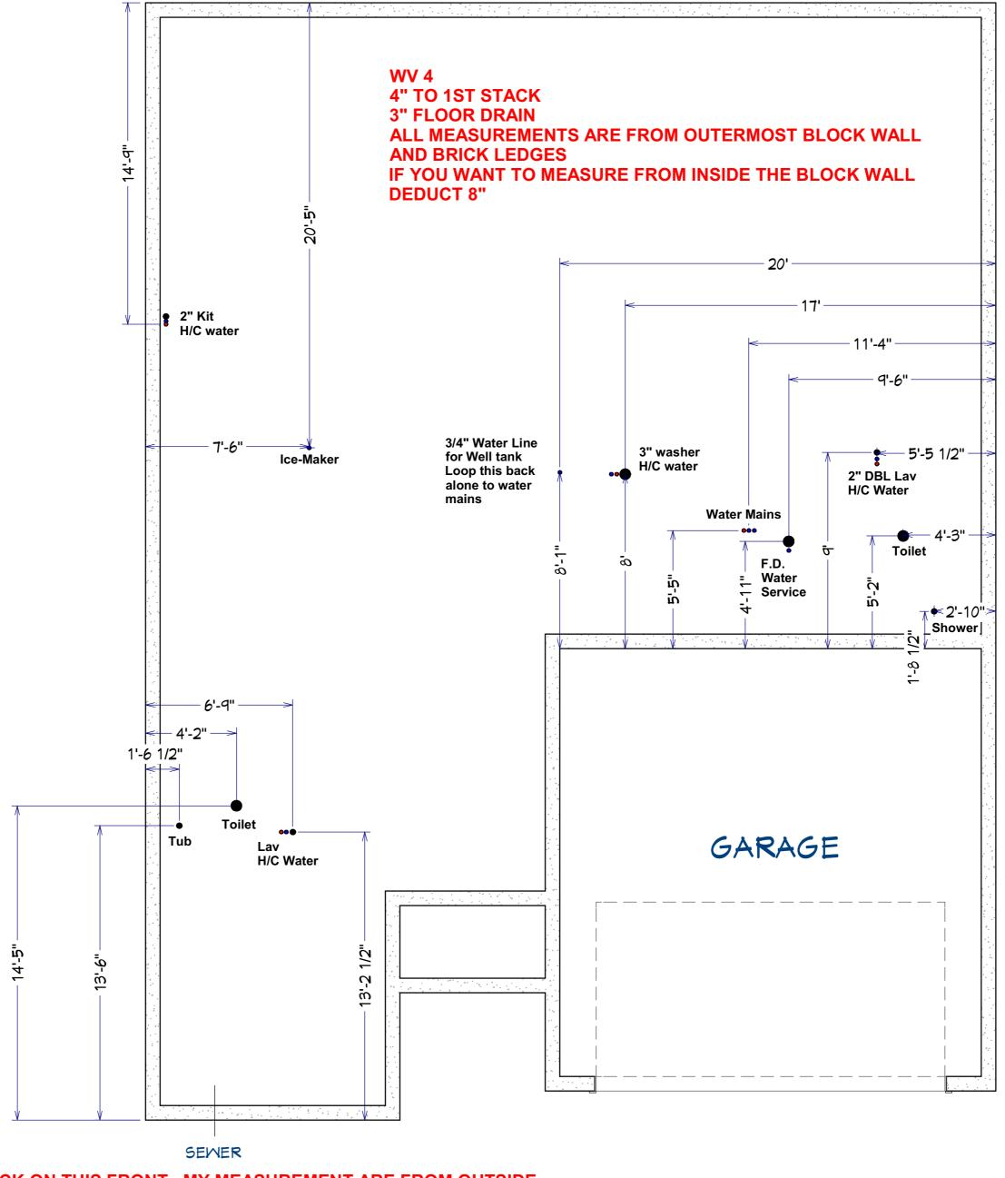
BRICK ON THIS FRONT, MY MEASUREMENT ARE FROM OUTSIDE OF BRICK LEDGE, DEDUCT 8" TO MEASURE FROM INSIDE BLOCK WALL
