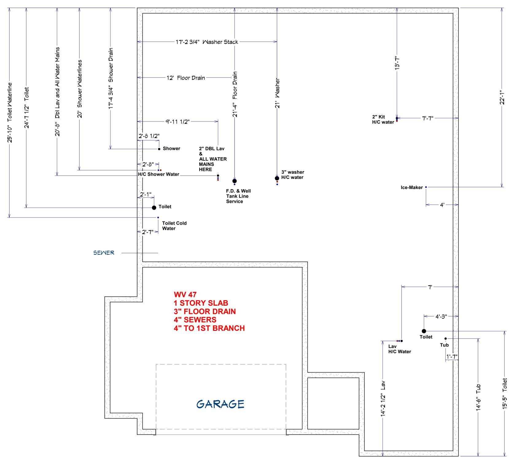
THESE MEASUREMENTS ARE FROM OUTERMOST PART OF FOUNDATION WALL, IF HAS A BRICK LEDGE THEN ACCOUNT FOR THAT AND PULL MEASUREMENT FROM OUTSIDE OF WALL. OR YOU CAN JUST DEDUCT 8" FROM MY MEASUREMENTS AND PULL FROM INSIDE THE BLOCK WALL.
